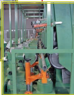
MOD. SF 3000/200/6U with 6 belt units Driving system of pieces to be worked: V-guides
