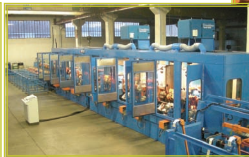
MOD. SF 3000/200/6U + CP 500/3U-200 with 6 belt units and 3 mop units Driving system of pieces to be worked: roller conveyor with pneumatic pinch-rolls
