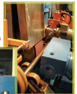
MOD. SF 3000/200/6U + CP 500/3U-200 with 6 belt units and 3 mop units Driving system of pieces to be worked: roller conveyor with pneumatic pinch-rolls
