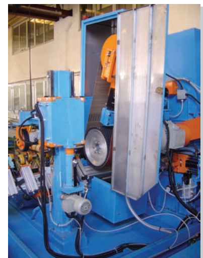
Detail of hood and inclined base
