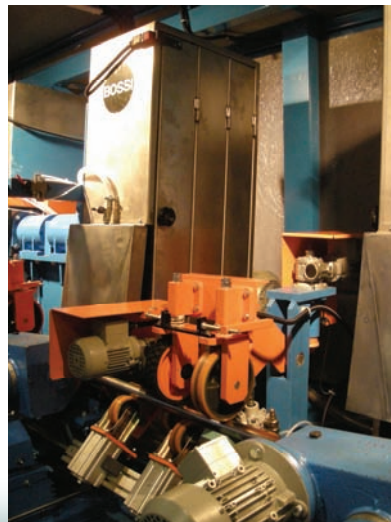
Detail of head and pinch-roll
