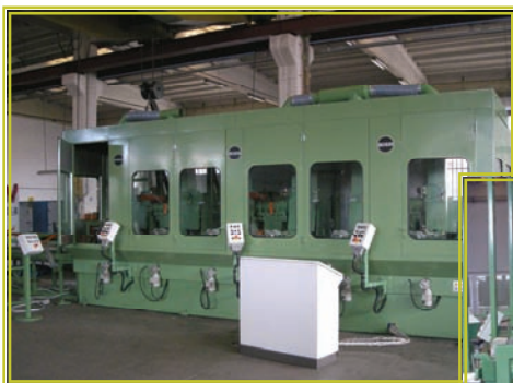
MOD. SF 3000/200/6U with 6 belt units Driving system of pieces to be worked: V-guides
